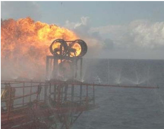
Photo: The semi-submersible drilling vessel 'NanHai II' owned by China Offshore Services Limited was used to drill Anambas-1X, AAL-2X-R and AAL-3X. Drill stem test (DST) - flaring activities.
