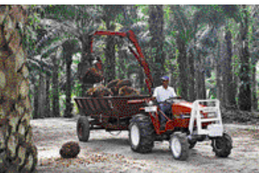
Mechanised FFB collection using the grabber
