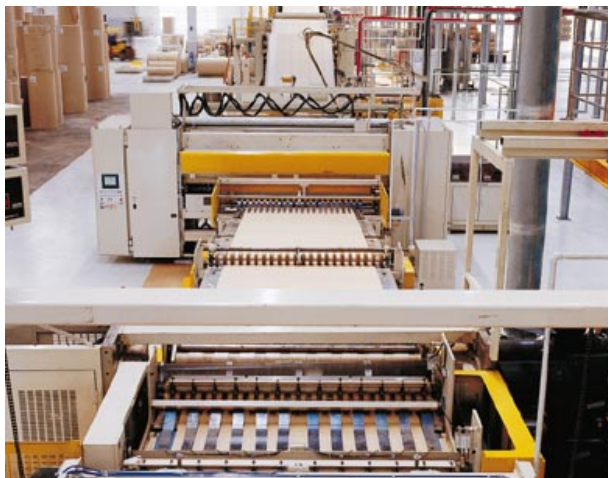
Genting Sanyen box plants feature the Mitsubishi Corrugator - one of the fastest corrugators in the world.
